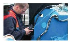
**Evaluating machine conditions** – Mobile vibration diagnosis, telemonitoring and telediagnosis, inspection and evaluation.
