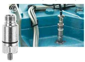
**VIBROWEB® XP** – Monitoring of critical machine trains with only a few measurement locations (low speed gears, compressors, wind turbines...)
